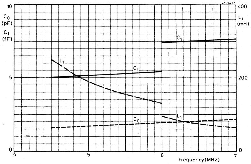
Fig. 6. Typical values of L_1 , C_0 and C_1 for frequencies from 4.5 to 7 MHz.
